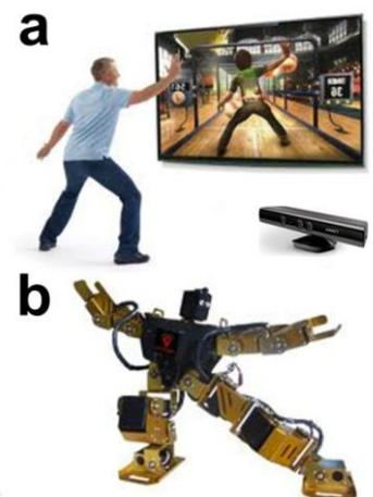
Fig. 2. (a) Motion detection using a *Kinect*. (b) A humanoid robot replicates the captured motion.
